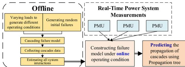
FIGURE 1. Development of a dynamic failure model for predicting cascades.
