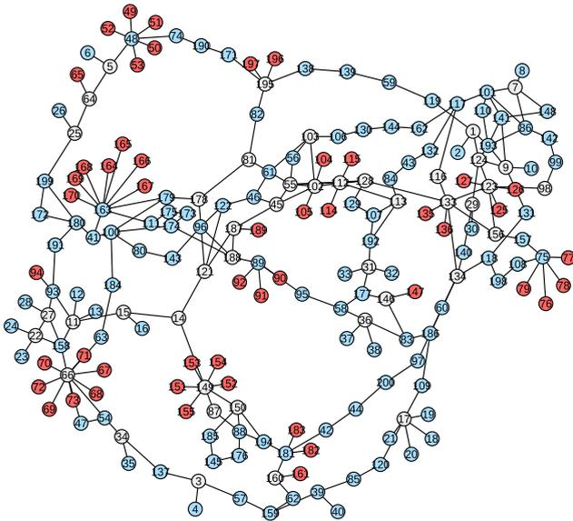
**FIGURE 6.** Diagram of Illinois 200-bus system that has 200 buses and 245 transmission lines. Red nodes represent generator buses and blue nodes represent load buses.
