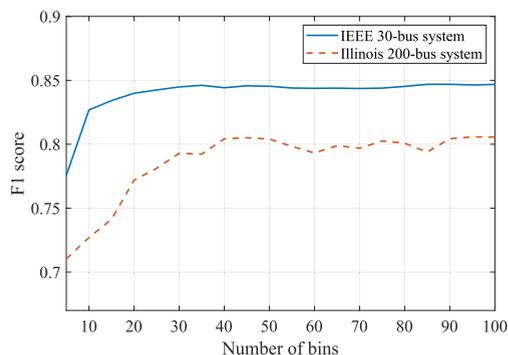
FIGURE 10.  $F_1$  score of prediction accuracy of total failures in IEEE 30-bus and Illinois 200-bus systems with different bins (from 1 to 100).
