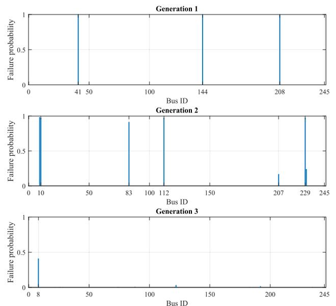
FIGURE 13. Potential failures in each generation of a cascade in Illinois 200-bus system.
