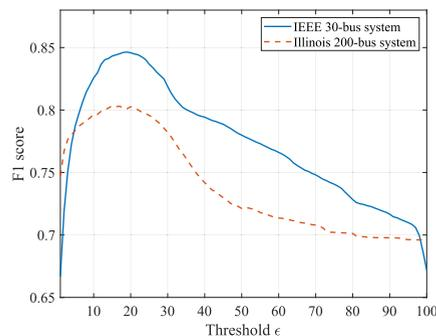
FIGURE 9.  $F_1$  score of prediction accuracy of total failures in IEEE 30-bus and Illinois systems with different  $\varepsilon \in [0, 1]$ .
