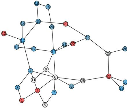
**FIGURE 5.** Diagram of IEEE 30-bus system that has 30 buses and 41 transmission lines. Red nodes represent generator buses and blue nodes represent load buses.
