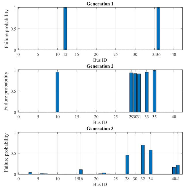
FIGURE 12. Potential failures in each generation of a cascade in IEEE 30-bus system.
